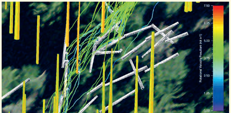
Standing (yellow/orange) and lying trees (white) influence the speed of the rolling stones (green in the image).
