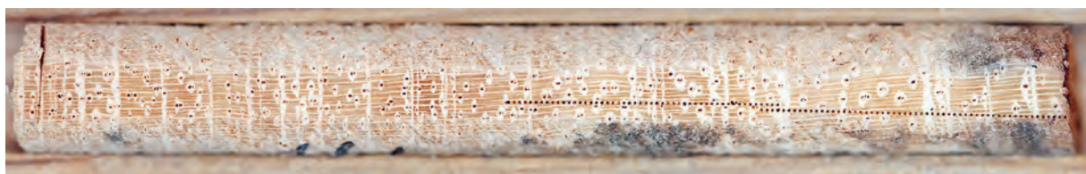
Wood from a Jatobá tree in Costa Rica. Bright lines and pores are clearly visible, as are the burn holes from the laser ablation device. The holes are in a neat row, each 0.1 millimetres in diameter.
