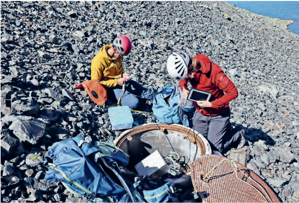
Temperatures are measured in mountain substrates in over thirty boreholes in the Swiss Alps.
