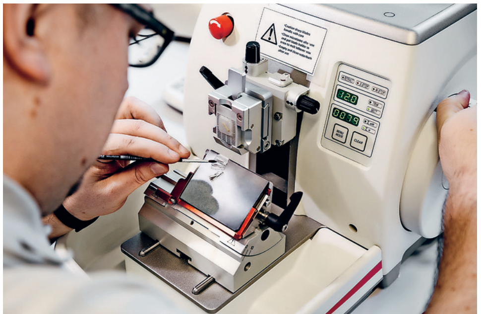
Cutting machine for fine things: with a so-called rotary microtome, Loïc Schneider produces wafer-thin slivers of the wood cores.
