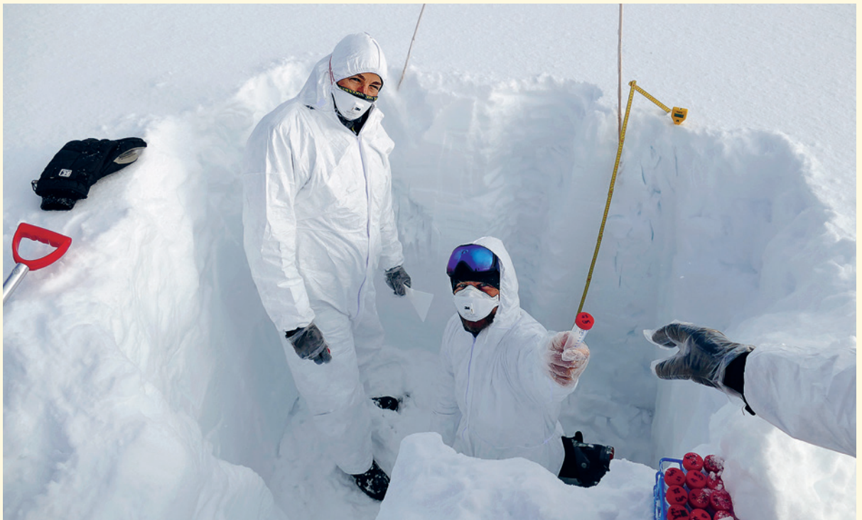
Taking samples at the Weissfluhjoch test site above Davos. To avoid contaminating the snow samples, the researchers wear protection suits and face masks.
