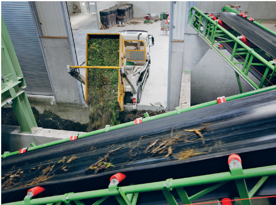
Collected organic waste is mulched into particles with a maximum size of 60 mm and fed into the biogas fermenter, where the industrial transformation of non-woody biomass into biogas takes place.
