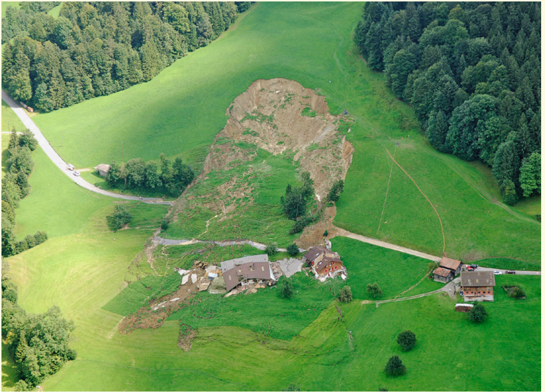
Plants can prevent landslides, but not in all cases: in pastures, for example, intensive grazing and fertilization can interfere with their stabilizing effect.
