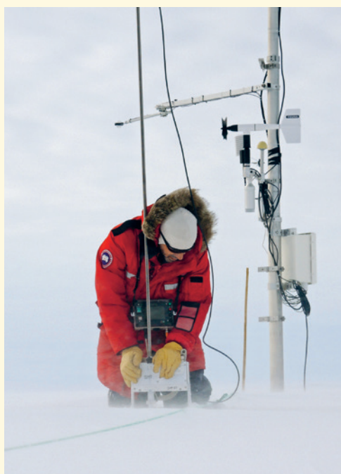
Martin Schneebeli examines the snow cover near a weather station using the SnowMicroPen.
