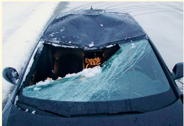
A chunk of snow that fell from the northern entrance of the San Bernardino Tunnel caused extensive damage to this vehicle.
