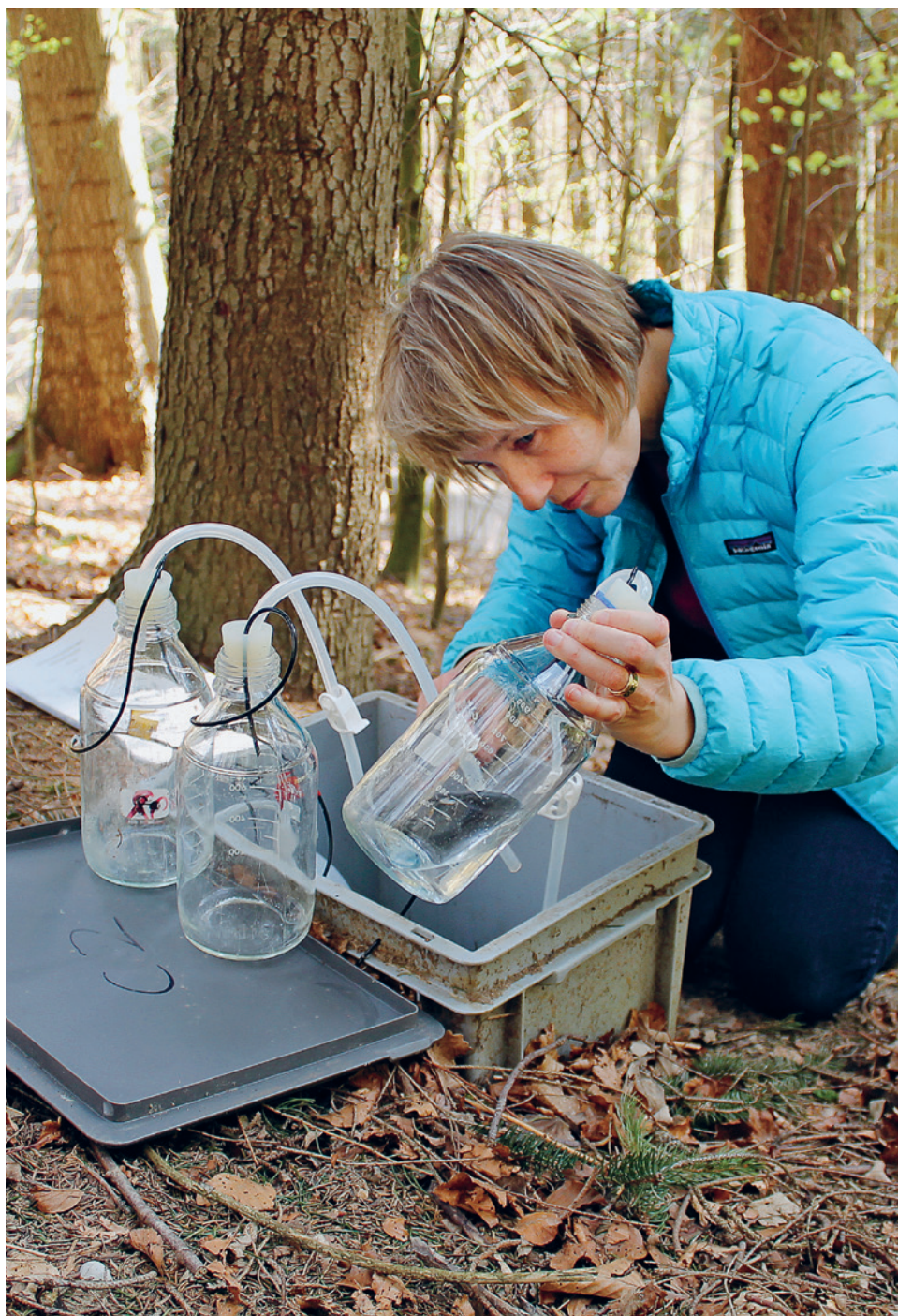
Elisabeth Graf Pannatier checks the volume of water sucked from the lysimeters.
