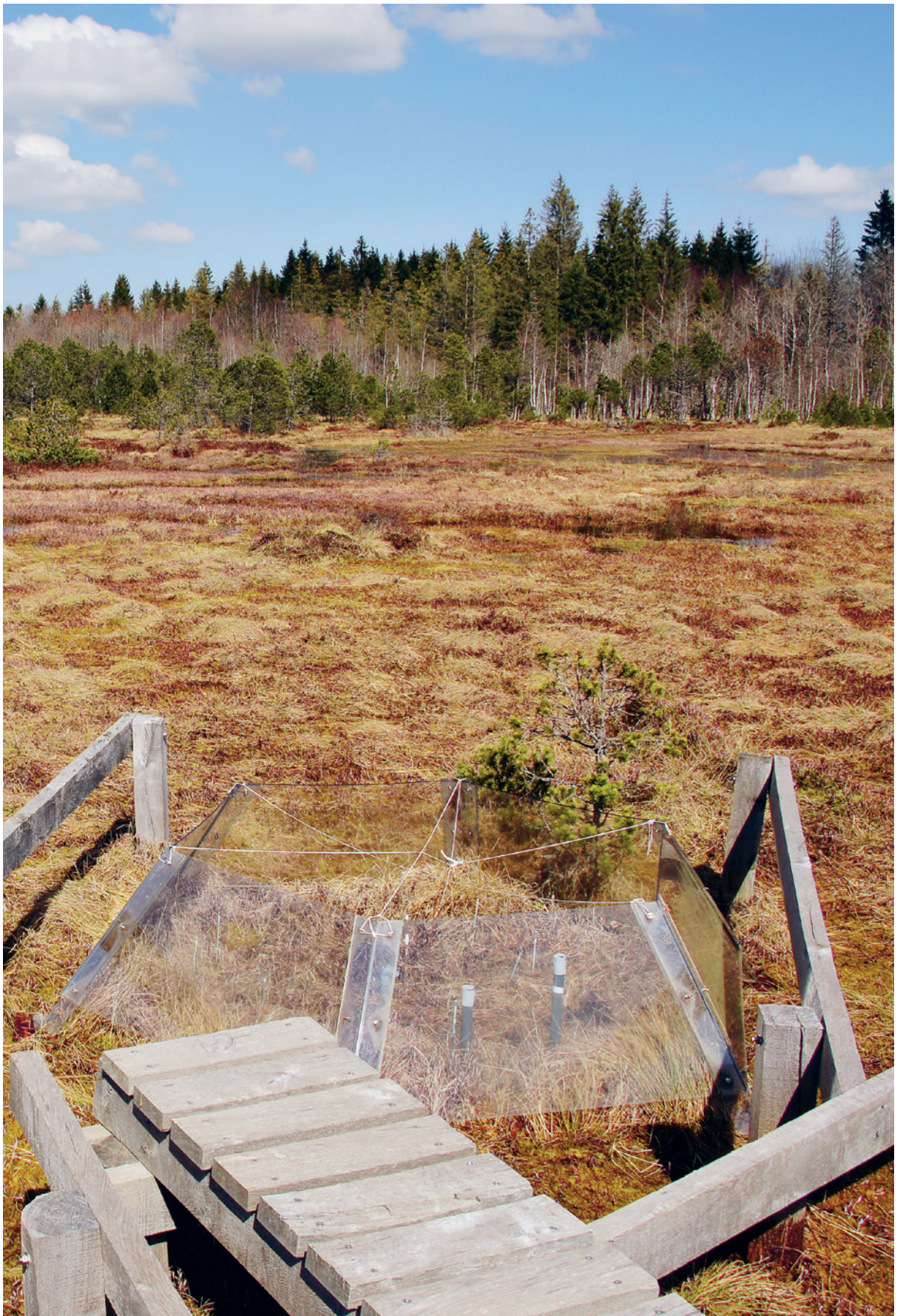
In the Le Forbonnet raised bog near Frasné in the Jura mountains of France, open top chambers simulate climate warming on a small scale.
