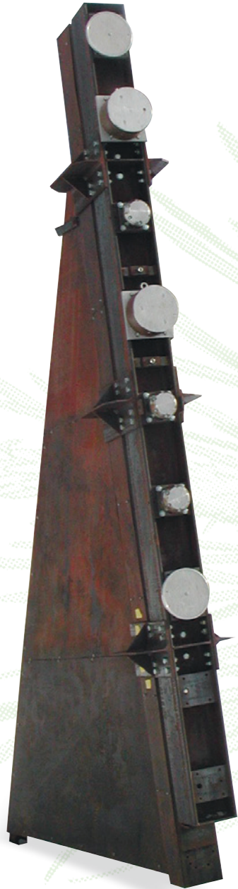
Instrumented steel wedge to measure avalanches
