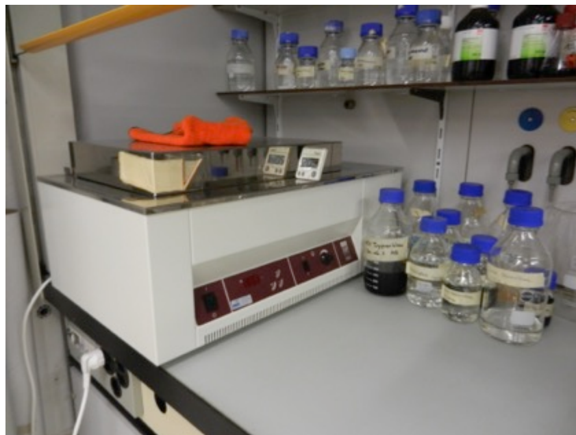
Figure 23: Water bath for the clearing and staining procedure of the roots.
