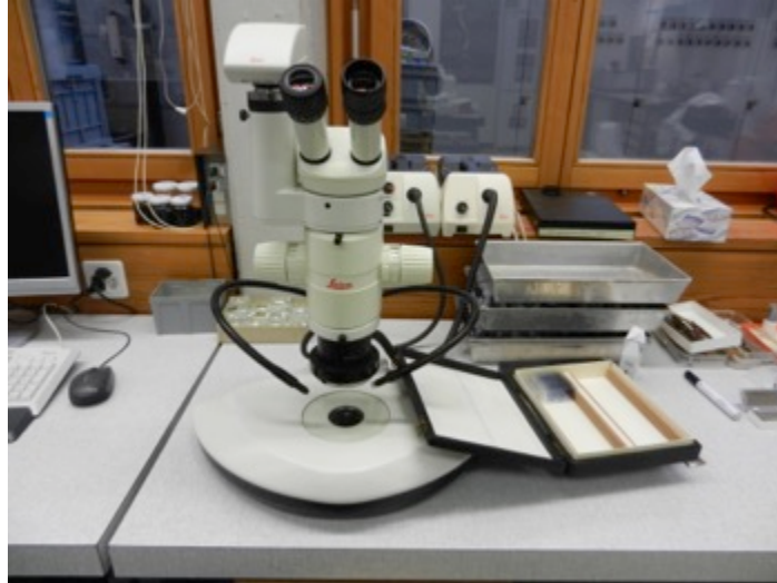
Figure 28: Stereo magnifier (Leitz Laborlux S) with Leica DFC 290 camera used to detect EMF.
