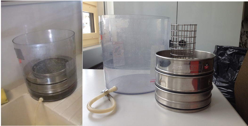
Figure 19: Wet-sieving analysis tools (left side: sieve tower in pot, right side: sieve tower with steel mesh cylinder).
