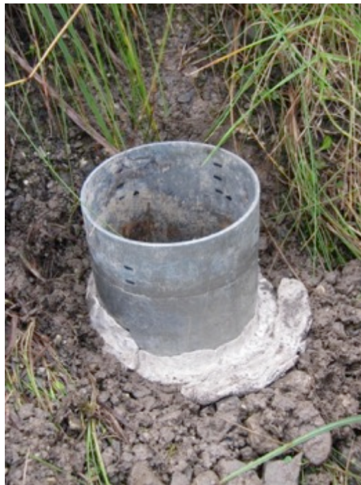
Figure 32: Experimental set-up for the permeability test (cylinder core sealed with plastic modeling mass).
