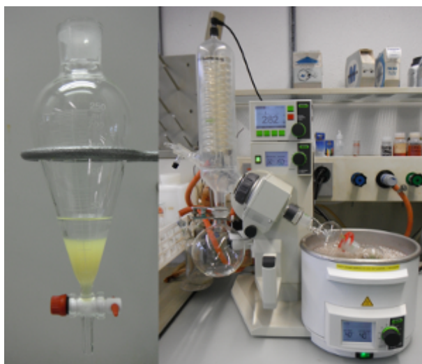
Figure 2.5: Left: Separation funnel with the transparent n-hexane layer on top and the yellow methanol-ethanol-KOH mixture at the bottom. Right: Vacuum dryer. Photo Bader A. 2013.
