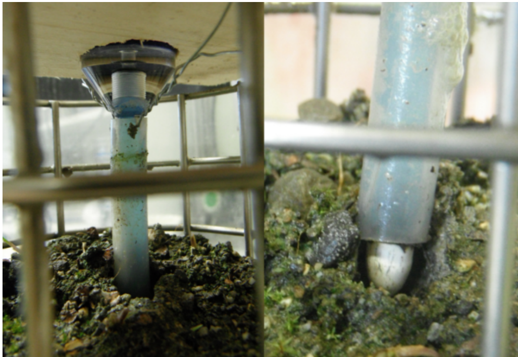
Figure 4.1: This figure illustrates the contact between the tensiometer cup and the surrounding soil after the wet-sieving procedure. Left: Sample AP2. Right: Sample AP4. Photo Bader A. 2013.
