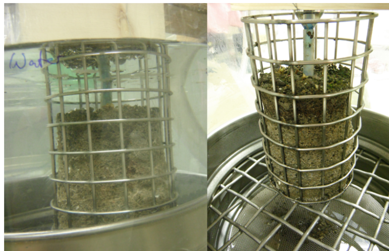
Figure 3.8: Wet-sieving procedure of the combined non-mycorrhized sample of Alnus incana and Poa pratensis (AP10). Left: During flooding. Right: After the wet-sieving the high grade porous ceramic cup of the tensiometer still remained in contact with the soil.
