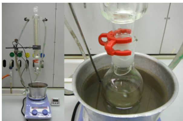
Figure 2.4: Saponification process of the Ergosterol liquid phase extraction. The round bottom flask was heated for 35 minutes in the oil bath adjusted to 110 °C and a speed of 1460 rpm. Photo Bader A. 2013.
