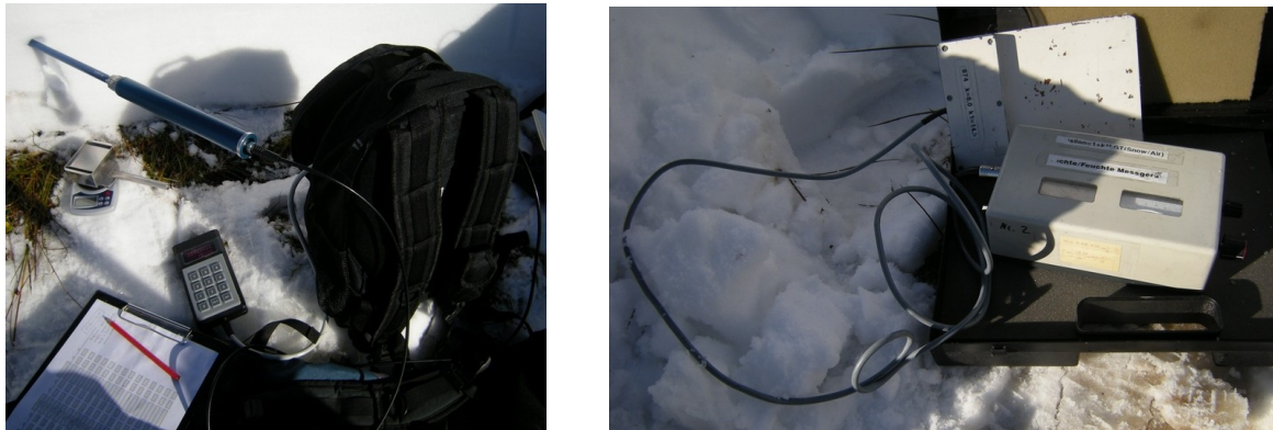
Figure 4.1: Snow Fork measuring device (left) and Denoth wetness meter (right). The Snow Fork consists of a battery box (hidden in the back-pack), the keyboard-display unit and the almost 1 m long steel fork. The Denoth tool has a plate-like sensor-unit and a control unit for manual tuning. Photos: Techel, 2009.
