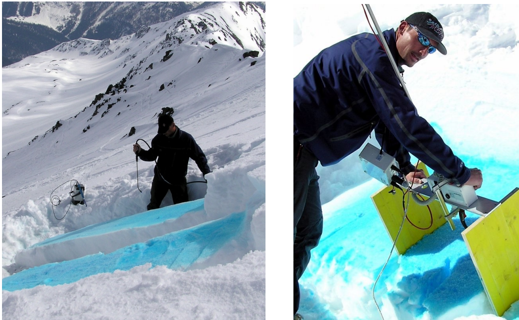
Figure 5.3: Left) artificial wetting of exposed layers using an ice-water-tracer mixture (Brilliant Blue food coloring). Right) SMP measurements. The SMP was mounted to a frame allowing easy positioning for measurements. Photos: Pielmeier, 2009, 2007
