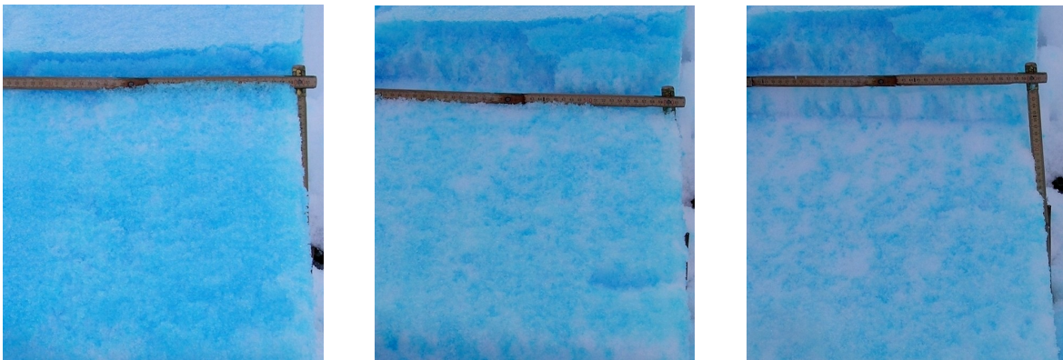
Figure 4.10: Water flow during artificial wetting experiments - persistent snow. The density of preferential flow channels was often high in layers consisting of coarse-grained persistent crystals. Surface layers showed matrix flow. Figure shows flow channel distribution at depths of 5, 15 and 25 cm below the surface (left to right, Weissfluh, Institutsgipfel, 2600 m, N, 38°, 10 April 2009). Photos: Pielmeier
