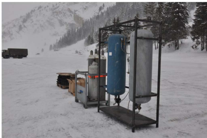
Fig. 2. Pressure reduction tanks for oxygen (blue) and propane (metallic). The gas bottles can be seen in the background. (For interpretation of the references to color in this figure legend, the reader is referred to the web version of this article.)
