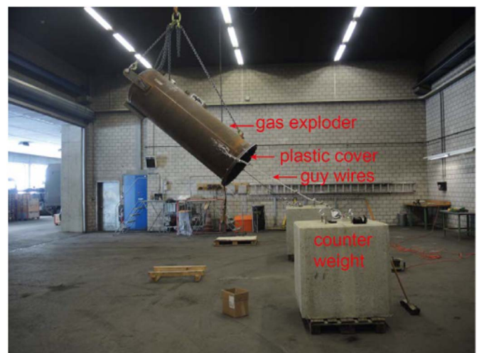
Fig. 1. View of the gas exploder, suspended from a crane. The pre-tensioned guy wires are connecting the gas exploder to the counterweights. The lower end of the tube is closed by a plastic cover.
