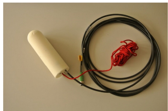
Fig. 2. Acceleration sensor sealed in foam cylinder (length: 20 cm, diameter: 6 cm).
