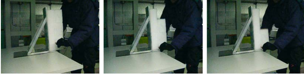
Figure 4. Series of pictures shot during a mode II fracture test. There is no visible opening of the crack. The mode I component was minimised by tilting the table by an angle \alpha \approx 5^\circ .
