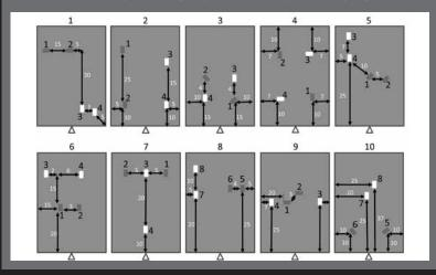
FIG. 2: SEARCH SCENARIOS IN THE TEST ON COL DU LAUTARET. SAME PRESENTATION AS IN FIG.1. ALL TRANSMITTERS ARE TURNED ON AT ALL TIMES. THE CIRCULAR TRANSMITTER SYMBOL INDICATES VERTICAL ANTENNA ORIENTATION.
