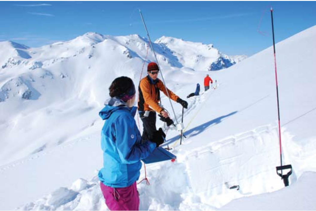
Field measurements on the fracture behavior of snow: performing series of PST in the course of a day and concurrently measuring slab stiffness with the SMP. Photo courtesy Jürg Schweizer
