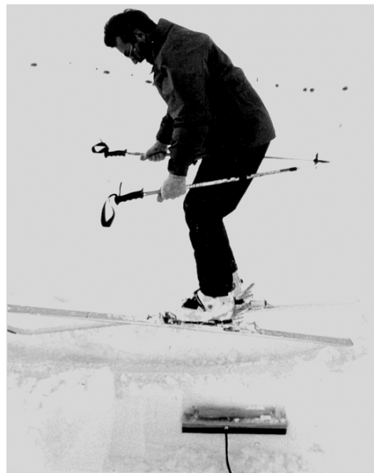
Fig. 2. Loading step of jumping; to show the configuration the load cell was partly dug out. The load cell was originally 32 cm below the snow surface, during jumping the distance between skier and load cell reduced to 11 cm. For scale: the load cell's dimension is 50 cm.
