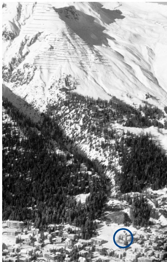
Figure 3. Snow Avalanche Path From the Schiahorn, Davos, Switzerland. Starting zone above, partly with supporting structures, avalanche track in narrow creek bed and run-out zone into residential area. In 1962, a disastrous avalanche was recorded in this path. The avalanche destroyed the forest just above the run-out zone (the gap is still visible) and damaged several houses in the run-out zone. The houses (circle) are the two only ones in the red zone (high hazard) where new buildings are prohibited. See Figure 4 for details of the hazard map (photo: Stefan Margreth, SLF).
