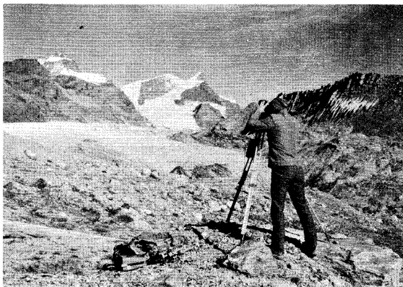
Figure E.7 Surveying of the former glacier bed of Findenlengletscher in 1987: Hermann Bösch operating the distance measurement instrument.
