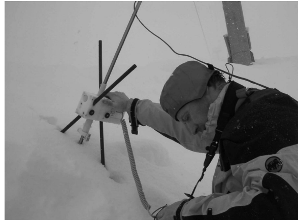
Figure 1: SMP profiling parallel to the manual snow profile and the stability test (Photo: SLF/A. Ræz).
