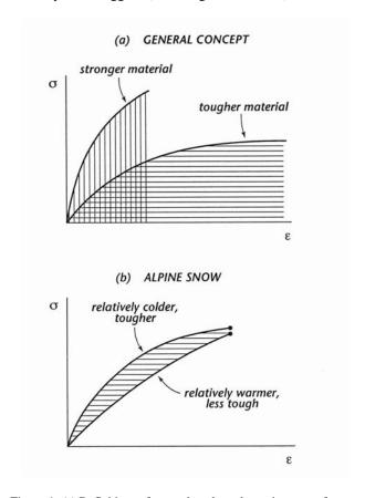
Figure 1: (a) Definitions of strength and toughness in terms of stress  $(\sigma)$  strain  $(\epsilon)$  curves. Strength is defined by the peak on the stress-strain curve. Toughness is defined as the area under the stress-strain curve until a peak is reached. Stiffness is defined as the initial slope of the stress-strain curve. (b) Schematic of stress-strain curves for alpine snow of two different temperatures: strength, toughness and stiffness decrease with increasing temperature.
