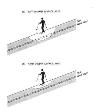
Figure 2: Schematic of influence (not to scale) of deformation imparted by a skier (a) for soft, warm slab properties (b) for hard, cold slab properties. In (a) deformation penetrates deeper whereas in (b) deformation does not penetrate as deep.
