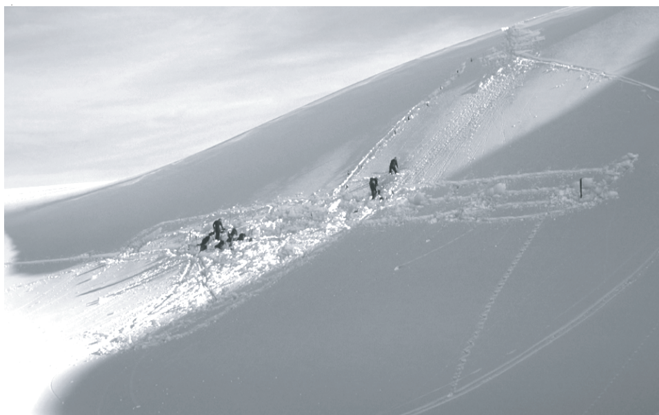
Fig. 2. The grid from 16 March 2001. Slope angles ranged from 20° in the lower part of the grid to 44° in the upper part. The upper arm of the grid is still not measured. Holes can be seen where the stuffblock test was carried out
