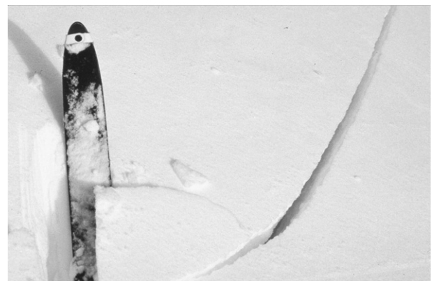
Fig. 2. Photograph of a crack that suddenly shoots out from a ski. This indicates the presence of a slab and weak layer both of which are favourable to skier-triggered slab avalanches.
