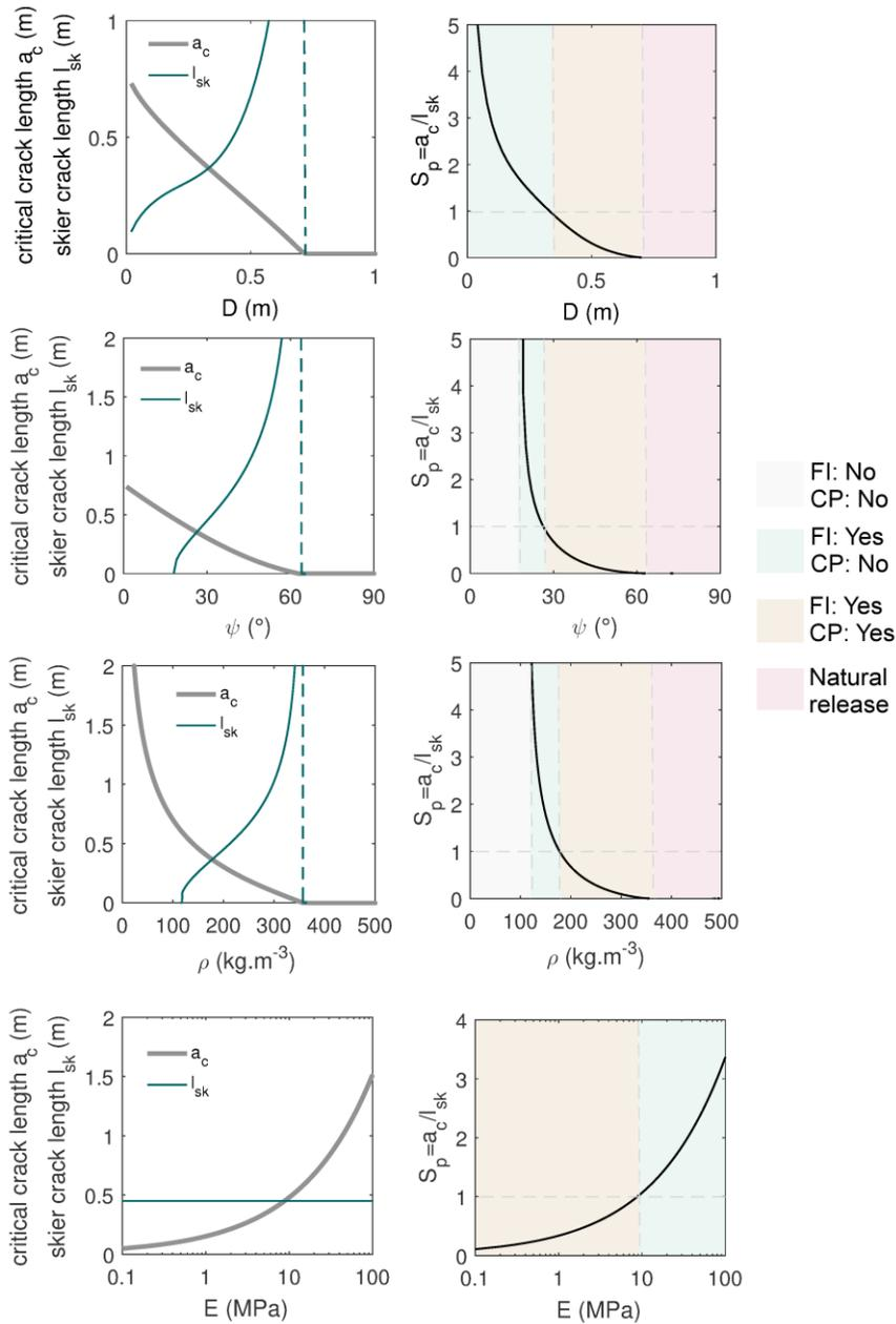
Fig. 4: Sensitivity analysis with independent snowpack properties, i.e. only one parameter was varied while the other properties were kept constant.  $D=0.4$  m,  $\psi = 30^\circ$ ,  $\rho=200$   $\text{kg m}^{-3}$ ,  $\tau_p = 700$  Pa,  $R=780$  N. FI: Failure initiation; CP: Crack propagation.
