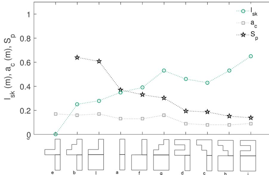
Fig. 6: Skier crack length, critical crack length and skier propagation index as a function of the profile type sorted to obtain a decreasing trend of  $S_p$ .
