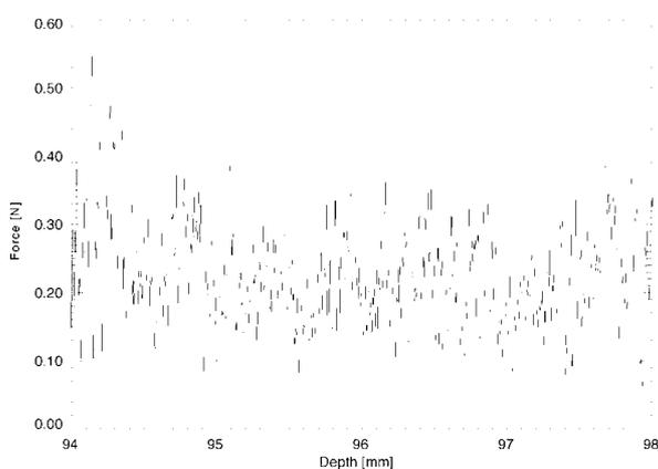
Fig. 2: Force signal measured in round-grained decomposed snow.
