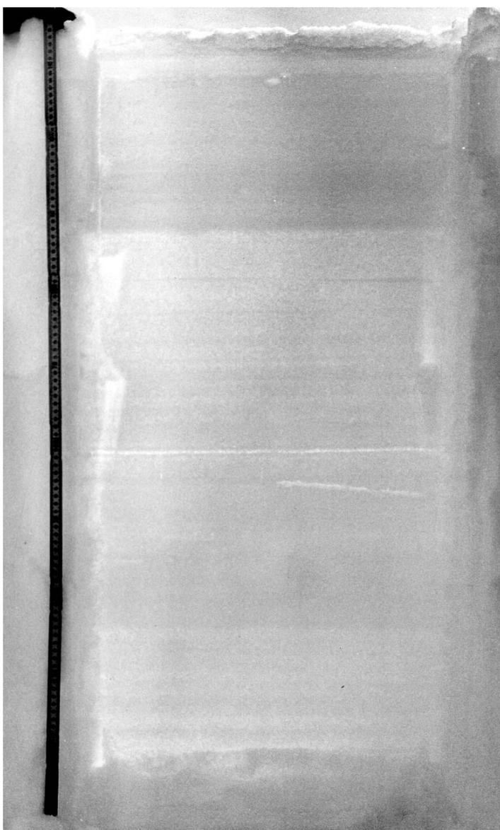
Fig. 20: Translucent profile with heated wire cutting, taken by Good and Krüsi (1992). The image analysis of these profiles produces as good results as stereological laboratory analysis and better results than the analysis of dyed profile images.
