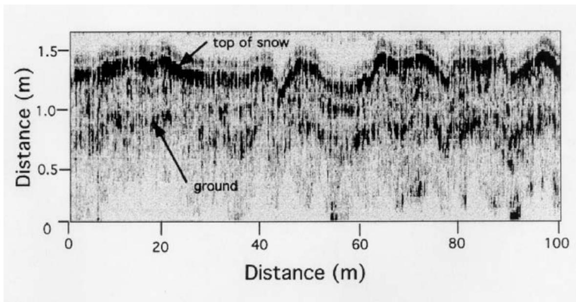
Fig. 22: FMCW radar profile of arctic snow pack (Holmgren, Sturm et al. 1998). It is not possible to resolve the complete snowpack stratigraphy. With higher resolution penetration depth and ground information are lost.
