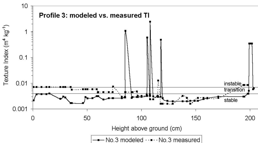
Fig. 7: TI comparison for profile 3.
