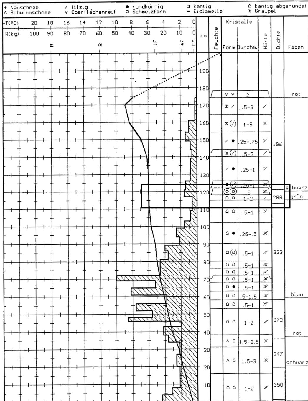
Fig. 11: Classical snow profile of test field profile. The profile section in comparison is contained in the black rectangle.
