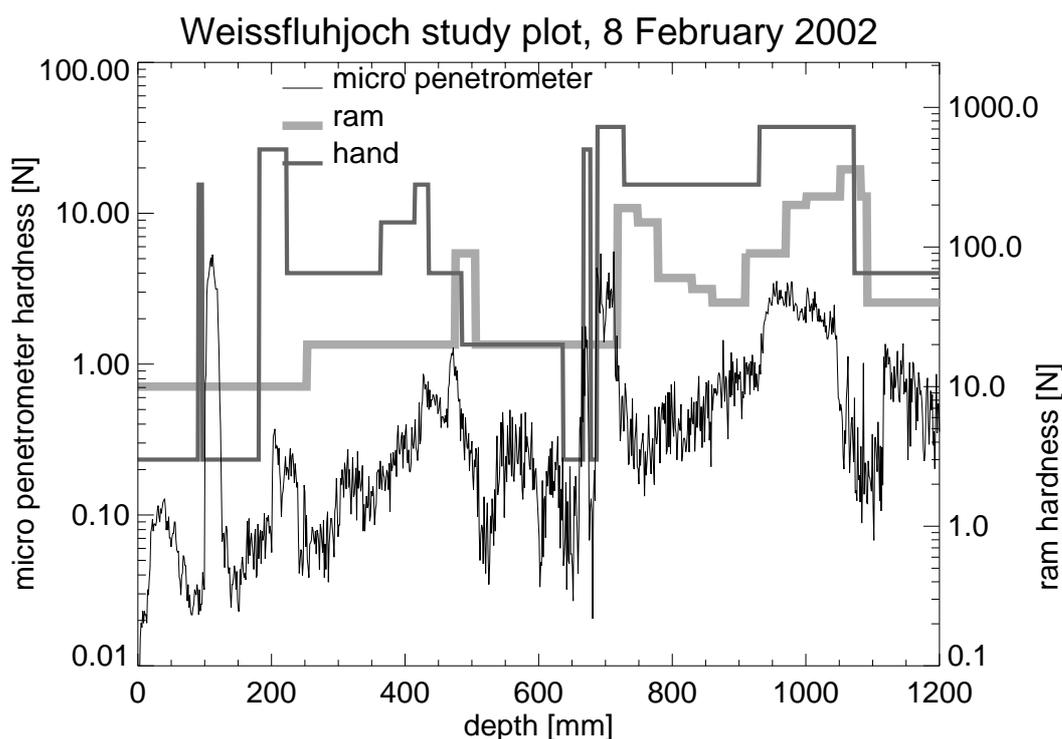
Fig. 25: Snow hardness measured by hand hardness and ramsonde (right y-axis) and by micro penetrometer (left y-axis, smoothed with moving average over 1 mm window). The logarithmic y-axes are chosen to get a better resolution in the lower hardness values. Differing in about one order of magnitude, the three hardness profiles can approximately be compared at these scales (Pielmeier and Schneebeli, 2002).
