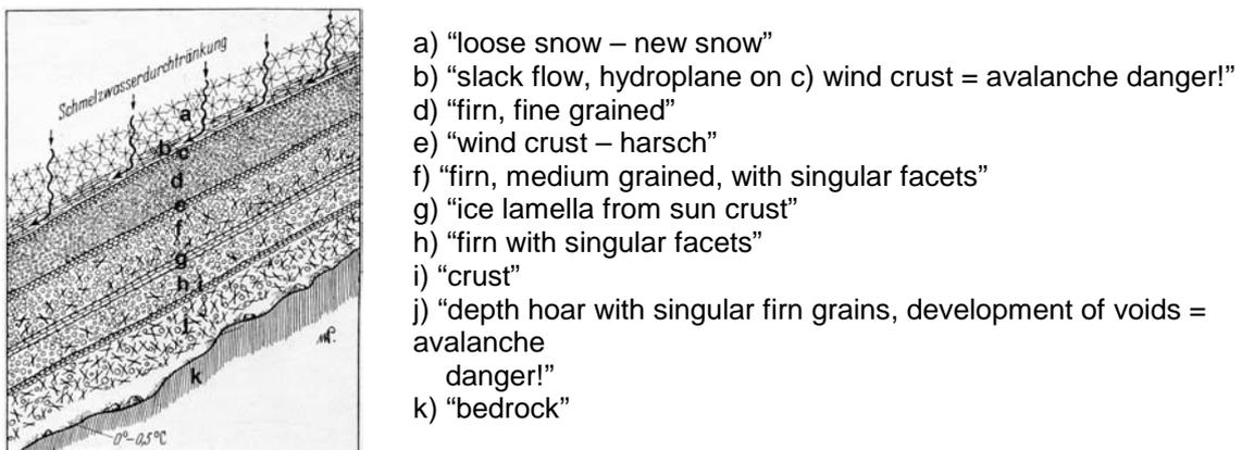
Fig. 4: Snow profile in the form a descriptive cross section of the snowpack (Paulcke, 1938)
