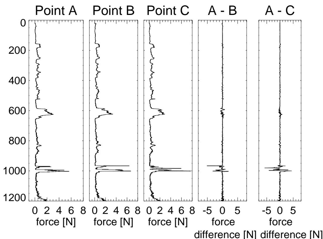
Fig. 1: Three micro penetrometer hardness profiles from the study plot Weissfluhjoch, Davos, point A, B and C with a spacing of 10 cm show the reproducibility of SMP measurements. Differences, A-B and A-C, occur at hard layers and crusts and are attributed to small-scale spatial variability of the snow properties in these layers.
