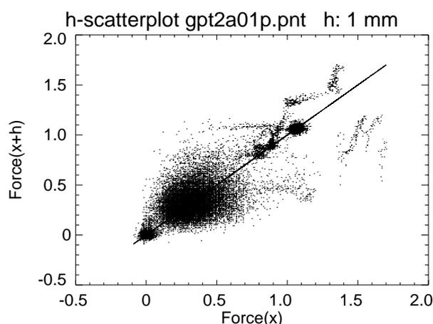
Fig. 4: H-scatterplot with a lag distance ( $h$ ) of 1 mm. It shows the spatial relationship of the force values at the location  $x$  to the force value at the location separated by the distance  $h$ .
