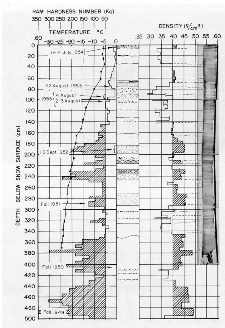
Fig. 13: Vertical snow stratigraphy and photo section (right). Strata of high and low density correlate with dark and light strata respectively on the photos. Layer boundaries are not always horizontal (Benson, 1969).
