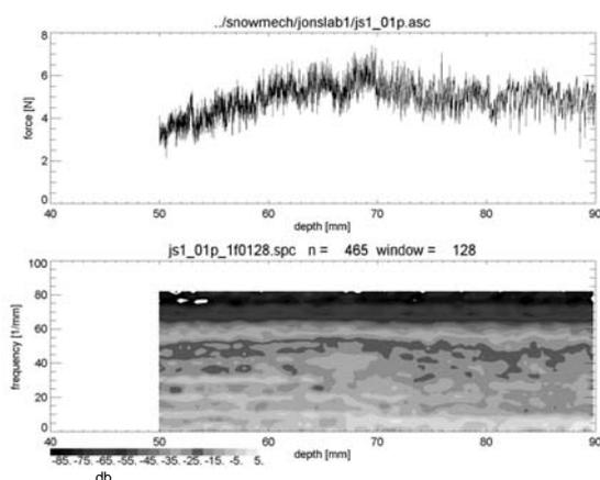
Fig. 9: Force signal and spectrum of a measurement where a failure occurred at depth 65 mm. The spectral bands seen above 65 mm disappear at this depth. Grey values show the intensities in decibel.
