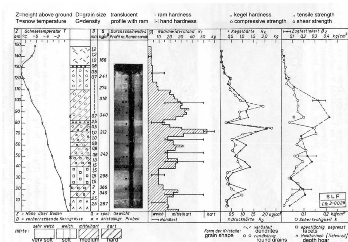
Fig. 12: Snow profile taken on 1 February 1950 with a translucent profile and a comparison of hardness measurements (De Quervain, 1950).
