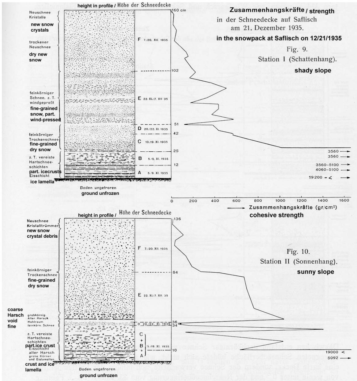
Fig. 7: Two snow profiles in terms of morphology and cohesive strength by Eugster (1938).
