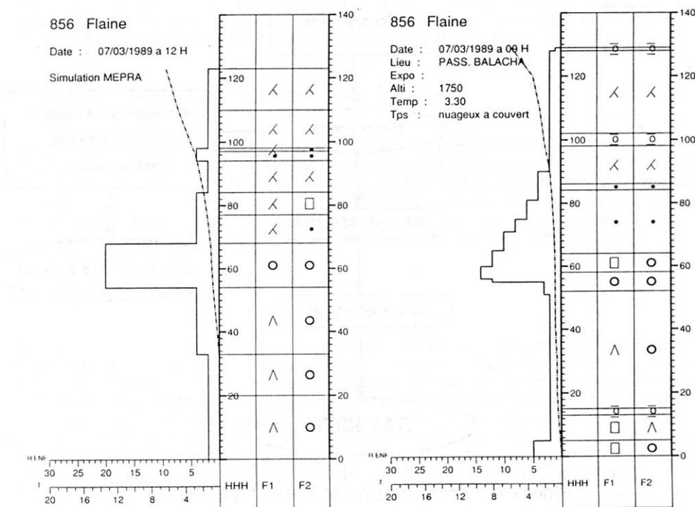
Fig. 23: Comparison of a MEPRA snow profile simulation (left) with a snow profile record (right) by Giraud (1992).
