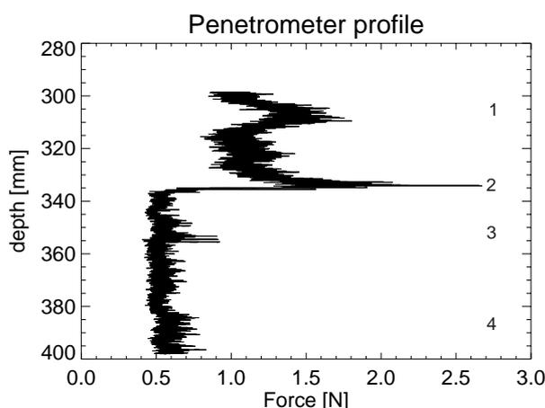
Fig. 10: Penetrometer signal of profile section. The positions of the numbers correspond to numbered layers in the translucent profile shown in Fig. 12.
