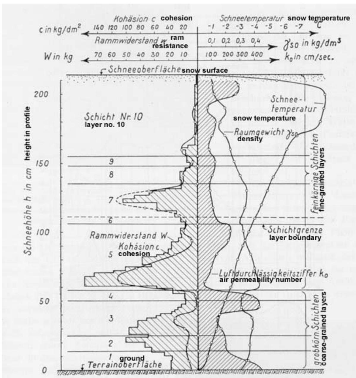
Fig. 9a: Complex snow profile taken by Haefeli on 16 February 1937 at the flat study plot Weissfluhjoch, Davos (Bader et al., 1939). Measured parameters are the stratigraphy based on the threads, ram resistance, cohesion, air permeability, density, snow temperature and grain size categories.
