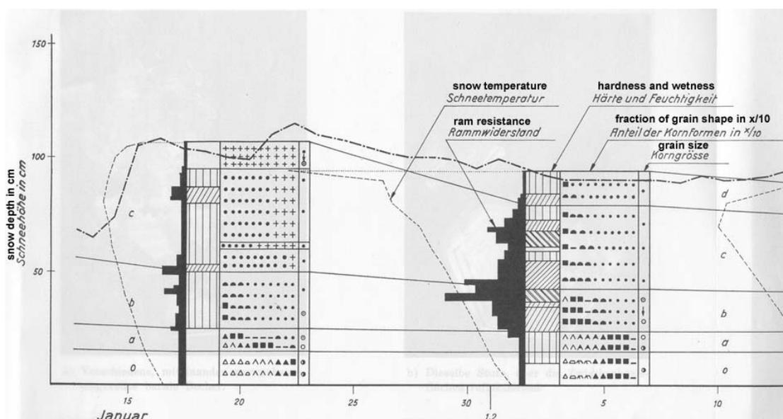
Fig. 14 Vertical snow profile section according to Eugster's (1952) expanded morphological classification where fractions (in tenths) of grain shapes are given for each layer.
