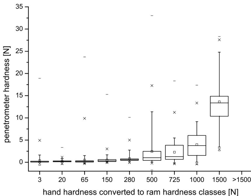
Fig. 10: Comparison of micro penetrometer hardness and hand hardness. Micro penetrometer hardness values in the respective ram hardness intervals are summarised in box charts. The box is determined by the 25th and 75th percentiles and the whiskers are determined by the 5th and 95th percentiles. The mean is indicated by the small square. First and 99th percentile are drawn as x and minimum and maximum as dash.
