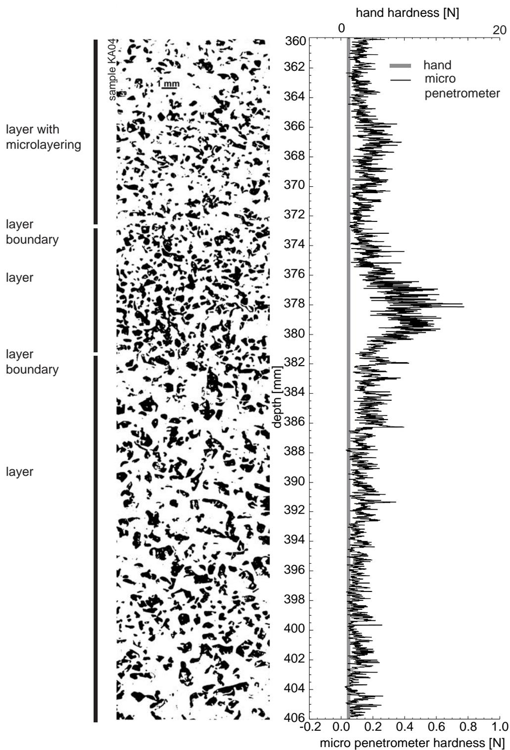
Fig. 4: Snow profile from 15 Jan. 2002: surface image containing thin, harder layer and micro layering (black is ice) and the corresponding hand and micro penetrometer hardness. This is an example where the stratigraphy established by hand hardness disagrees with the surface image because the thin, harder layer is missing.
