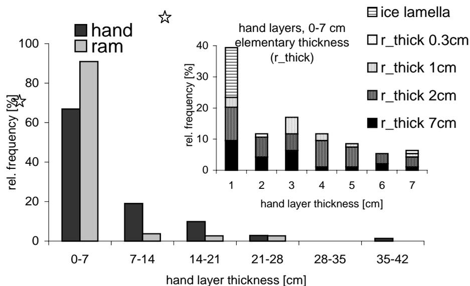
Fig. 7: Occurrences of layer thickness in ram and hand profiles. The inset shows the occurrences of hand layer thickness from 0-7 cm. The elementary thickness is the minimal layer thickness needed to perform the according hand hardness test (fist is 7 cm, 4 or 1 fingers is 2 cm, pencil is 1 cm, knife is 0.3 cm).
