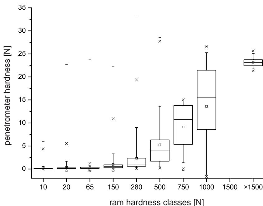
Fig. 9: Comparison of micro penetrometer hardness and ram hardness. Micro penetrometer hardness values in the respective ram hardness intervals are summarised in box charts. The box is determined by the 25th and 75th percentiles and the whiskers are determined by the 5th and 95th percentiles. The mean is indicated by the small square. First and 99th percentile are drawn as x and minimum and maximum as dash.
