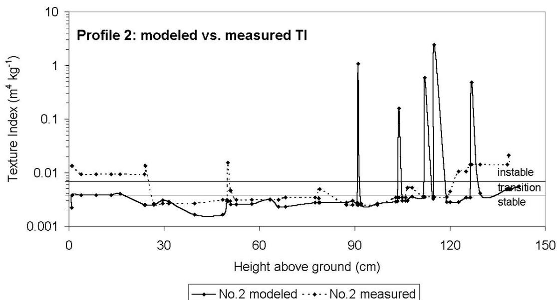
Fig. 5: TI comparison for profile 2.
