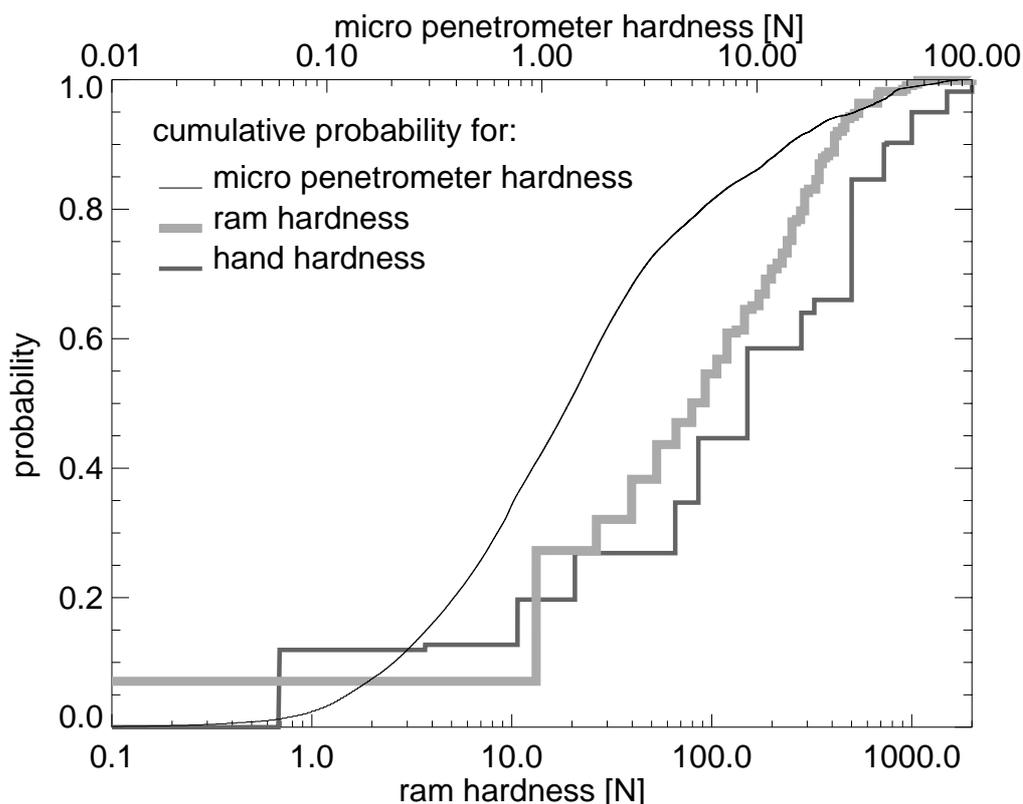
Fig. 8: Cumulative probability for ram hardness, hand hardness and micro penetrometer hardness on logarithmic x-axes. High hardness values occur with a greater probability in ram and hand hardness profiles than in micro penetrometer profiles.
