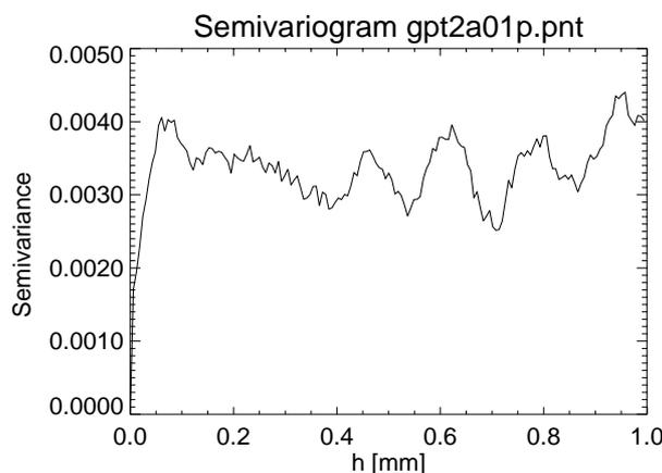
Fig. 5: Semivariogram showing spatial continuity up to a lag distance of 0.075 mm.
