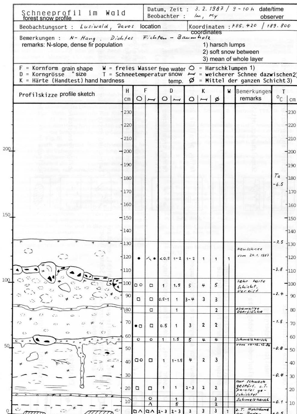
Fig. 16: Forest snow profile with a 2-dimensional profile sketch. A method developed and used by Imbeck (1987). The great variability in the profile and the not parallel layering required new morphological classes and more differentiations in layer boundaries.
