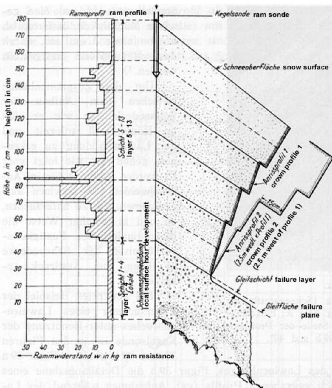
Fig. 9b: Complex slope profile taken by Haefeli above an avalanche crown (Bader et al., 1939). Measured parameters are the stratigraphy based hardness differences, ram resistance. Grain size and morphology are relative because they are only drawn.
