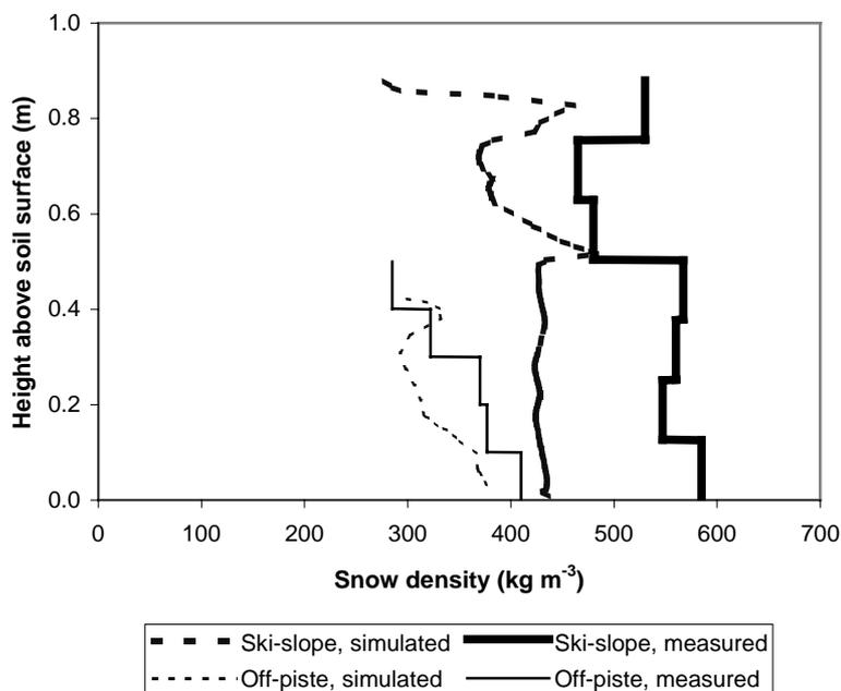
Fig. 6: Simulated and measured profiles of snow density at the Haggenegg ski-slope and off-piste site on 12 January.
