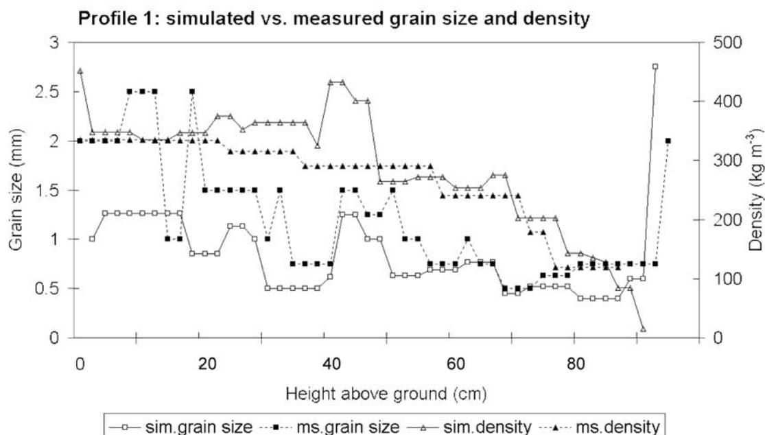
Fig. 4: Grain size and density for profile 1.
