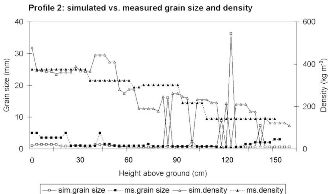
Fig. 6: Grain size and density for profile 2.
