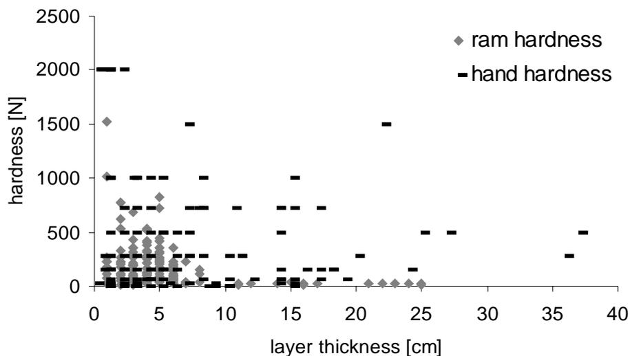
Fig. 6: The hand and ram hardness levels according to layer thickness. Ram hardness has a trend to more thin hard and thick soft layers, whereas hand hardness and thickness are more evenly spread.
