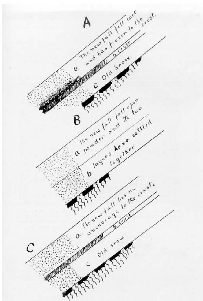
Fig. 6: "In A the NEW SNOW *a* fell wet and froze on to the CRUST LAYER *b*. It is therefore well anchored to it. A photograph of this state of affairs is shown in Fig. 5. In B the NEW FALL *a* fell upon POWDER SNOW *b* and the two have settled together. In C the NEW FALL *a* fell at low temperatures and has no anchorage to the CRUST LAYER *b* on which it lies. (Seligman, 1936, p. 309)
