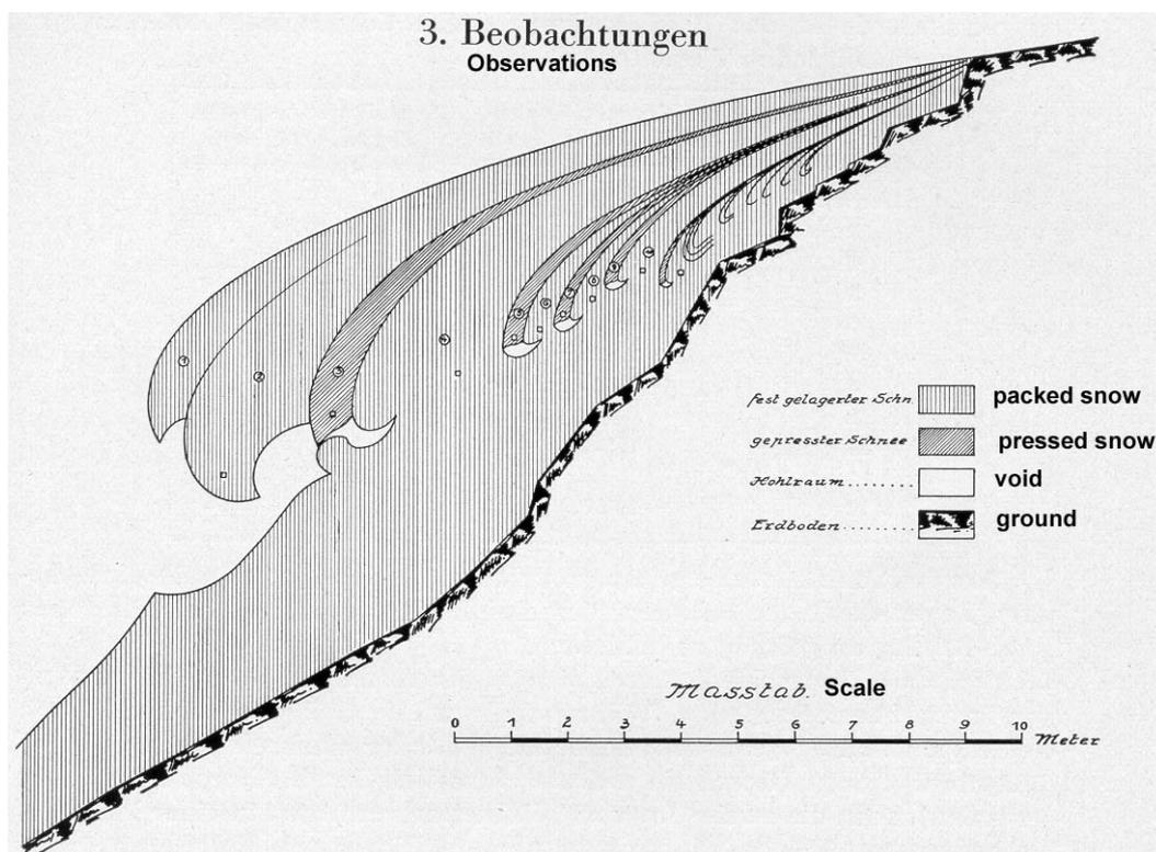
Fig. 2: Two-dimensional snow profile of a cornice drawn by Welzenbach (1930). The stratigraphy (layers 1-12) was established by density measurements.
