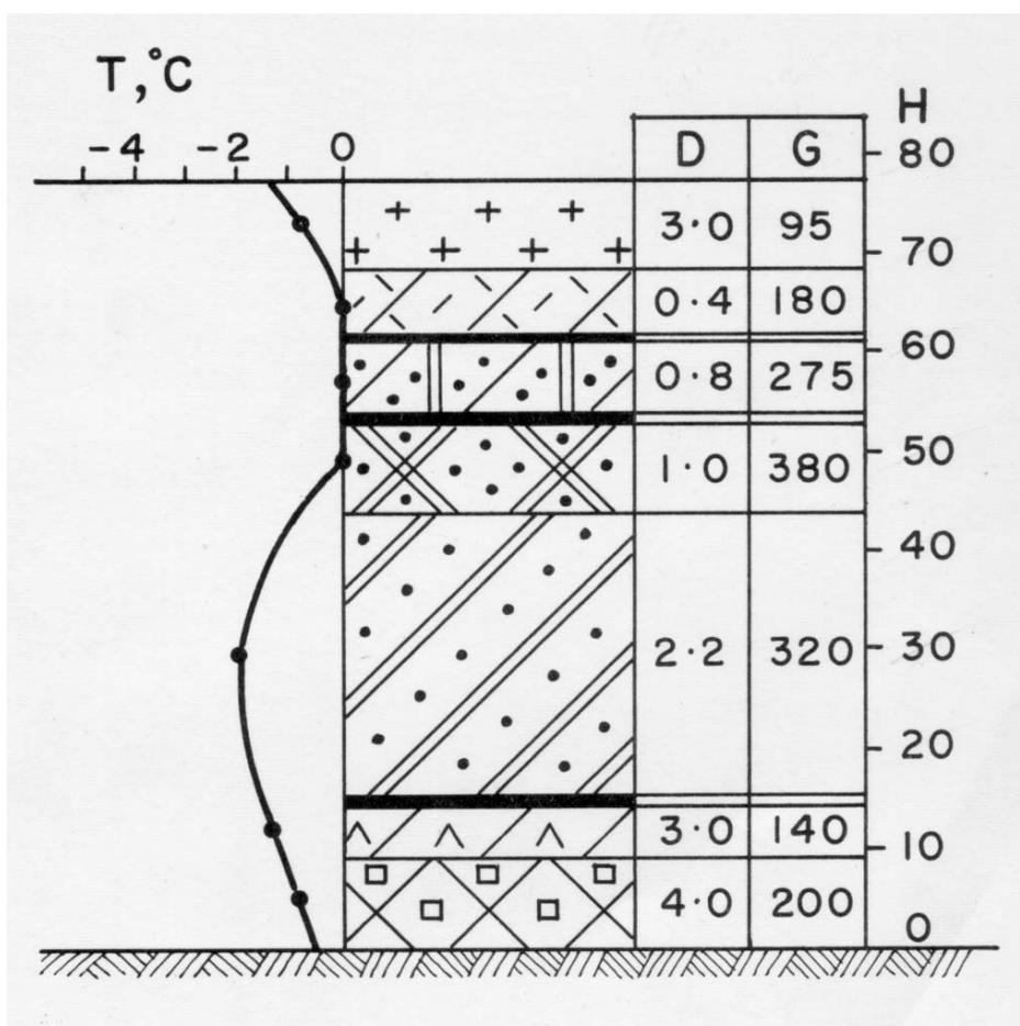
Fig. 15: Vertical snow profile section according to the International Snow Classification (Schaefer, Klein et al., 1954)
