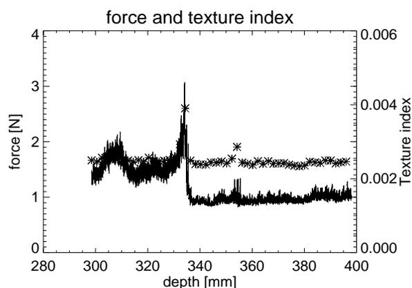
Fig. 8: Penetrometer force signal and texture index (asterisks) of a section of a natural snow profile .
