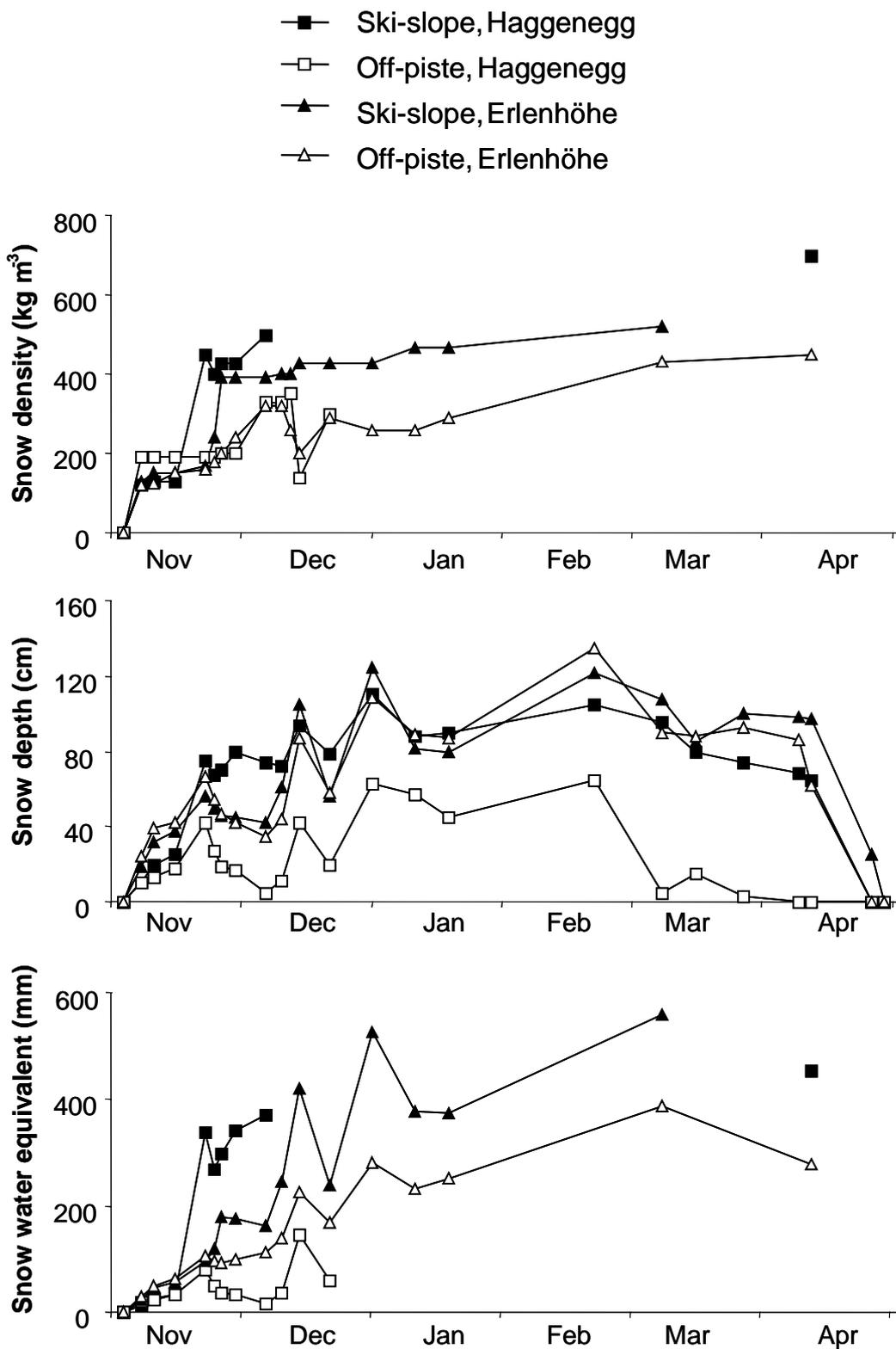
Fig. 1: Measured snow depth (cm), snow density ( $\text{kg m}^{-3}$ ) and snow water equivalent (mm) for the 4 locations during winter 1999/2000.
