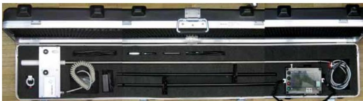
Figure 12: Transportation box for SMP with standard rod (1250 mm).
