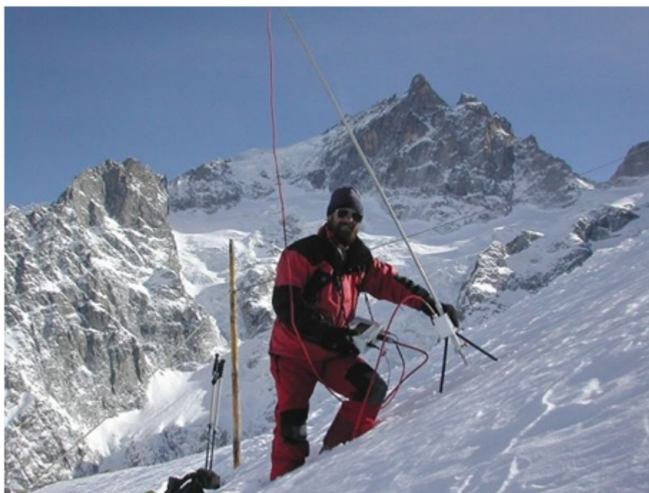
Figure 6: Correct measurement setup. The SMP is held perpendicular to the slope.
