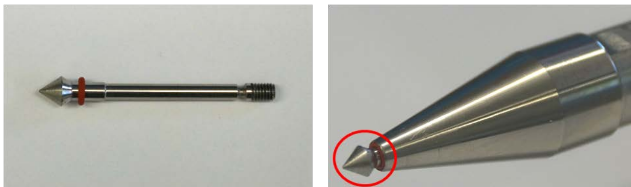
Figure 7: Measurement tip of the SnowMicroPen with O-ring.
