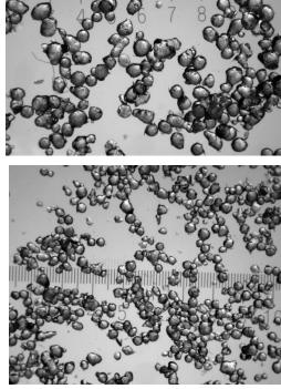
of machine made snow of different grain size and wetness
